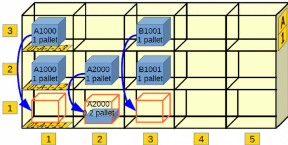
Replenishment strategy can be used to refill easily-reached locations in a warehouse system. In this example warehouse, the locations on the first level (01-A-1-\*1) are reachable by every warehouse worker, but higher levels (01-A-1-\*2, 3) are only reachable by fork lifts.
