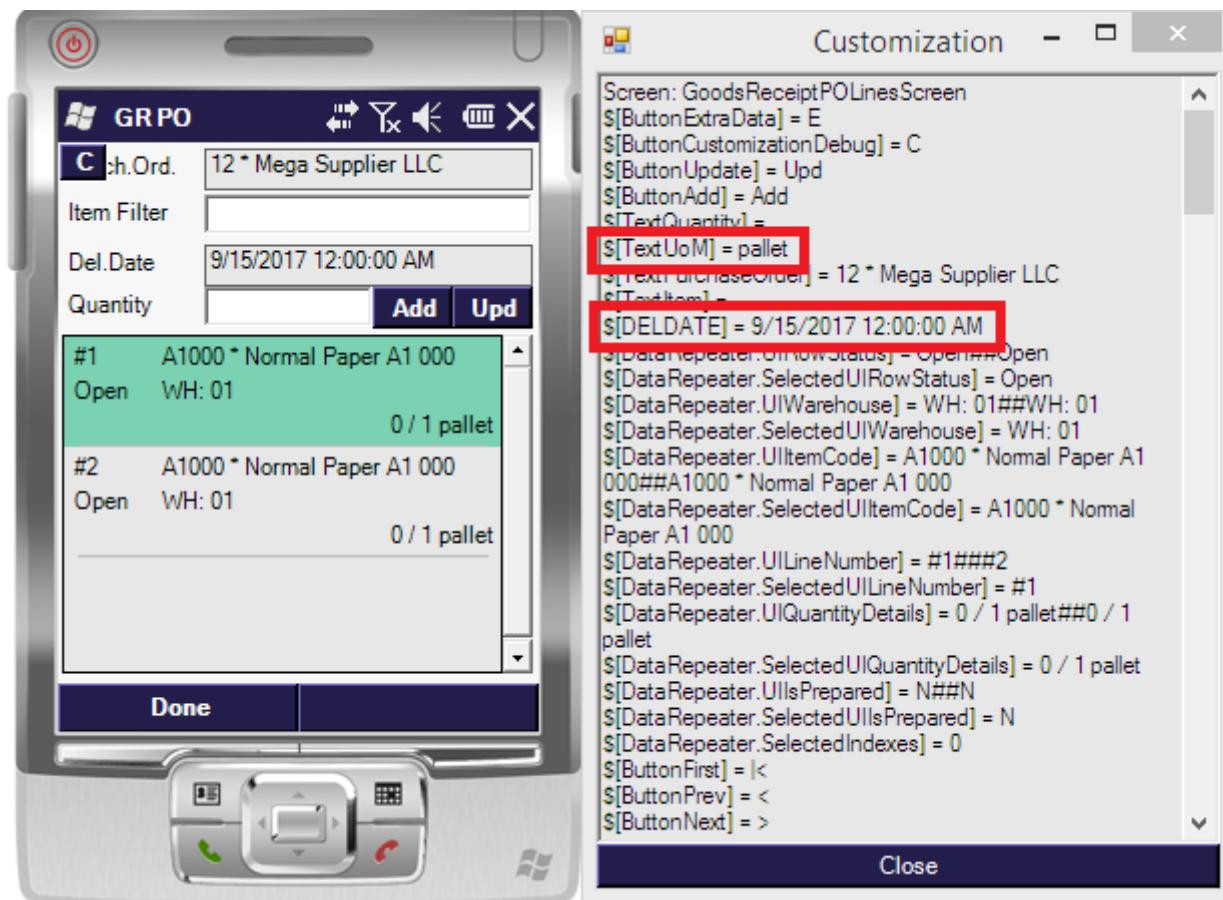
It is also possible to add fields that already exist in SAP Business One as a user defined field. In this case no user query is required to copy the values added on the scanner to the database, but additional user queries are needed to populate the fields on the device with the database values.
