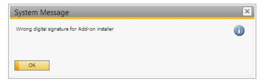
The most likely cause for this issue is that the installation .exe file was corrupted during the extraction process. Extract the installation .zip folder again and start the installation afresh.
