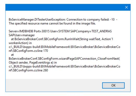
It means that the connection cannot be established to the database server. Go back to the Database connection screen of the Service Broker installer and enter the name of the database server with the exact same format as it was defined during the installation of the SAP Business One client.
