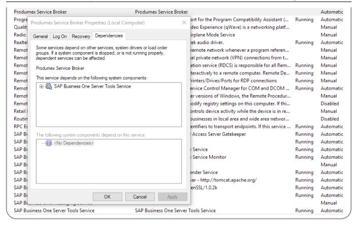
Please note: Do not set the dependency on HANA environments. Since the Produmex Service Broker is a Windows service, SAP HANA and Produmex Service Broker are running on separate servers. In order to avoid this issue, make sure that the HANA server is already running when you restart the server of the Service Broker.
