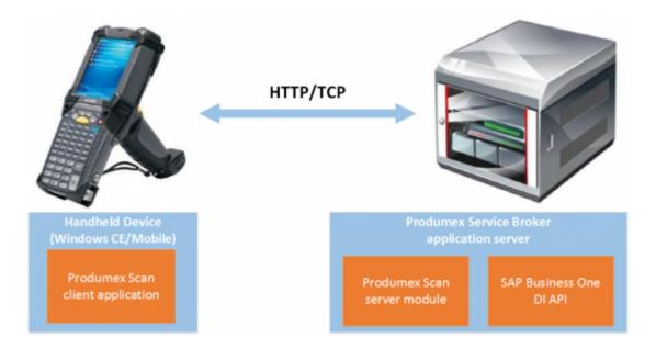
The add-on must be installed in SAP Business One. It is used mainly for set-up and administrative purposes; it does not need to be running for the mobile devices to work.
