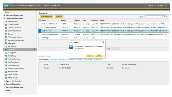
If the installation is successful, on the opening Synchronization Report the status on the line of Produmex Scan is 'Successful'. The installation zip is automatically moved to the Produmex Shared Repository folder.
