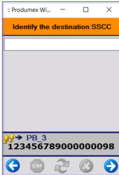
It is possible, through custom development, that multiple boxes are prepared for one pick list. If there are multiple boxes and it is not exactly defined what needs to be stored in which box, you will see a list of SSCC's on the screen and you need to scan one of them.
