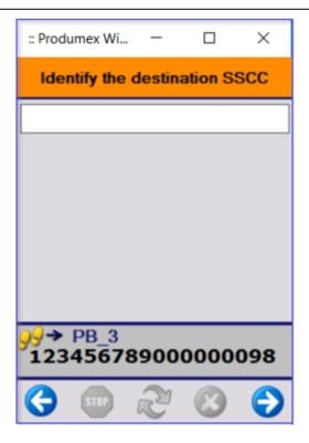
It is possible, through custom development, that multiple boxes are prepared for one pick list. If there are multiple boxes and it is not exactly defined what needs to be stored in which box, you will see a list of SSCC's on the screen and you need to scan one of them.
