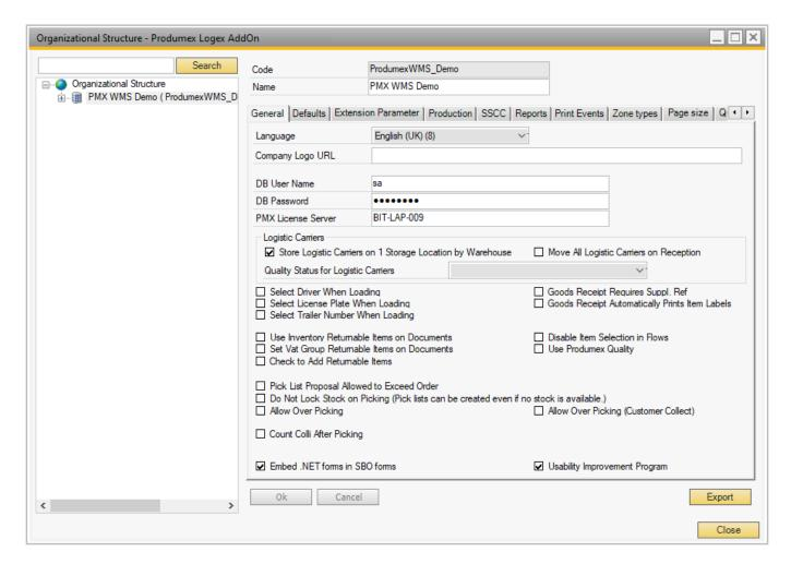
3. Make sure the IP address or host name of the server where the PMX License Server is running is filled in, add-on clients will require this to be able to connect.
