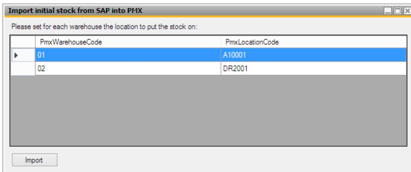
Enter the location code to the PmxLocationCode field on the line of the warehouse. Only active locations that belong to the warehouse can be added. If you leave the location code empty, the import is not performed for the given warehouse.
